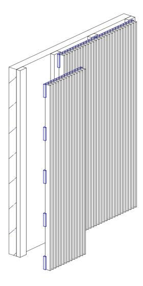
Panels are Secured to the Wall directly to Selected Wall Battens. Screw Fix through Face of Black Cross Members.
